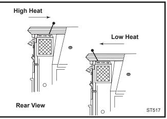
**Fig. 19** The thermostat handle may be positioned anywhere between the two extremes for different heat levels.
